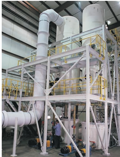
Dual stage HCl scrubber with fiberglass columns and catwalks.
