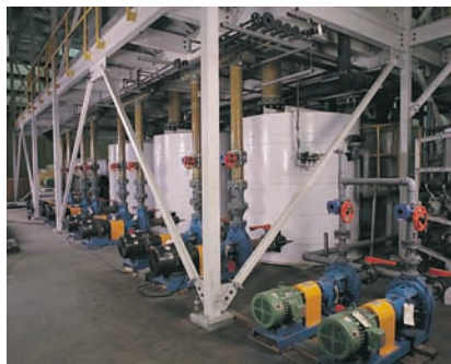
Multi-stage external recirculation system.
