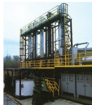
Tri-NO x Multi-Stage Multi-Chem system with acid recovery.
