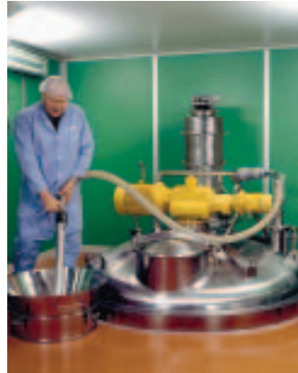
In a vacuum conveying system, the conveying is fully sealed off from the surrounding environment, which means a working environment without heavy lifting, dust or other contaminations.
