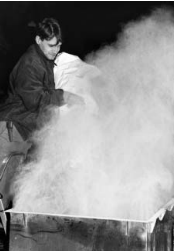
In manual handling the operators are subjected to heavy lifts and dusty premises.
