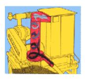
Centrifugal separator draws material into circular chamber where it spins out of air stream. Partially cleaned air rises up stack to...
