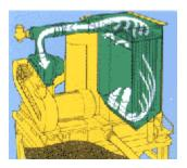
Final cloth dust collector, which filters out virtually all sub-micron particles. Cleaned air passes to vacuum pump and is exhausted through silencer.
