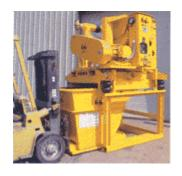
Full hoppers are removed by forklift and carried to the dump site. Two hoppers can be used for almost continuous operation.
