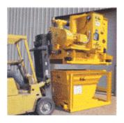
or conveniently lift just the "Powerhead" for transport to different hoppers throughout the plant.
