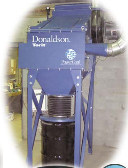
Torit PowerCore CPC-3 on clay and cement blending at a concrete block plant.
